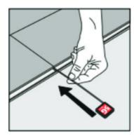
Make sure to insert the wire between the clip and the groove of the plank. Push the wire forward using the handle. **Step 2**Make sure you unlock the system.
