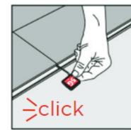
When the wire is inserted, move it slightly to hear the lock system disengage.
